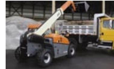
Material buckets help you load and unload loose materials quickly and easily.
